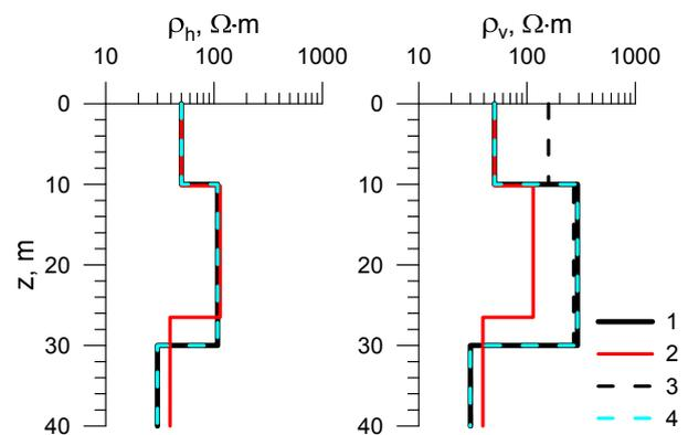
**Figure 3.** Results of different inversion procedures applications. 1 – base model, 2 – result of isotropic inversion of  $\rho_a^{xy}$  and  $\varphi_z^{xy}$ , 3 – anisotropic inversion of  $\rho_a^{xy}$ ,  $|T_{zy}|$ ,  $\varphi_z^{xy}$  and  $\varphi_T^{zy}$ , 4 – anisotropic inversion of  $\rho_a^{xy}$ ,  $|T_{zy}|$ ,  $\varphi_z^{xy}$  and  $\varphi_T^{zy}$  with  $\rho_v$  resolution analysis.
