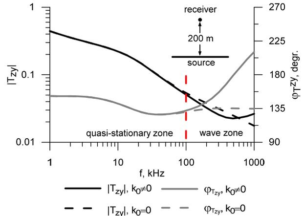
**Figure 1.** Comparison of tipper calculated with (solid lines) and without (dashed lines) accounting of the displacement currents in the air. Model is shown in Figure 2.
