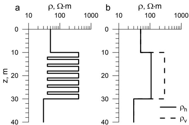
**Figure 2.** Base multilayer isotropic model (a) and equivalent anisotropic model (b).
