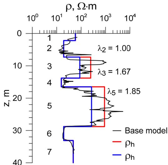
**Figure 4.** Result of the anisotropic inversion of synthetic CSRMT data compared with base electric logging diagram.
