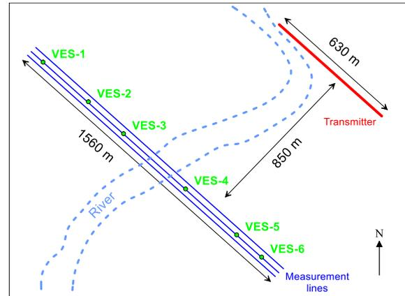
**Figure 1.** Configuration of the CSRMT survey area. Green dots indicate points of VES.
