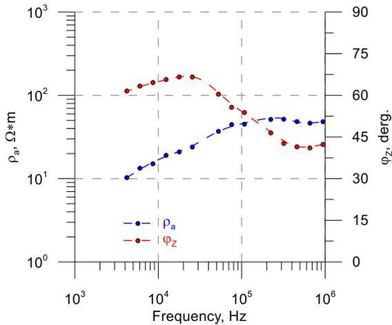
**Figure 2.** Example of the CSRMT sounding curves – apparent resistivity and impedance phase.
