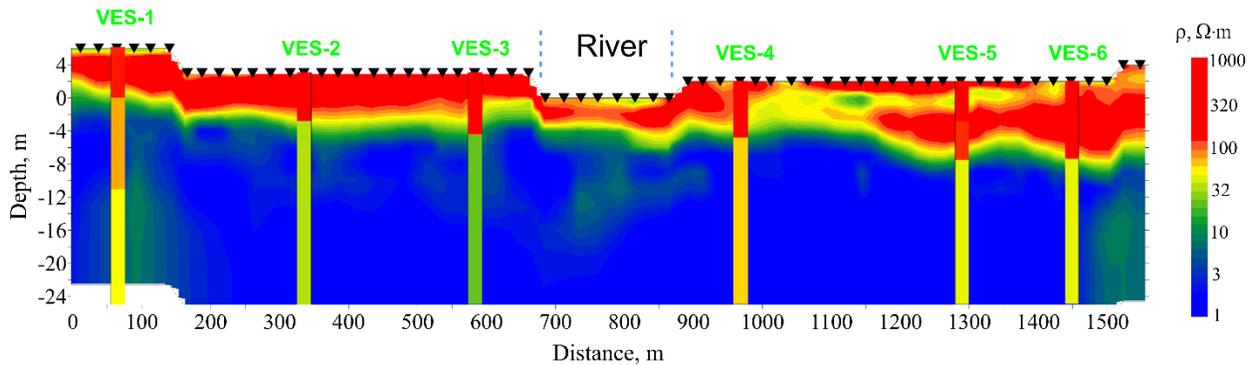
**Figure 3.** Results of 2D inversion of CSRMT data. Color columns represent results of 1D inversion of VES data. Black triangles indicate CSRMT measurement points.
